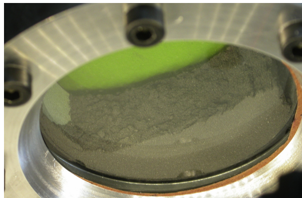
Fig. 1 – Picture of the rotating drum with an activated \text{LaNi}_5 sample inside.
