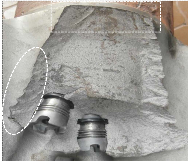
Fig. 3. Fracture surface of failed 8,5" oil well drill bit: initiation sites at the top.
