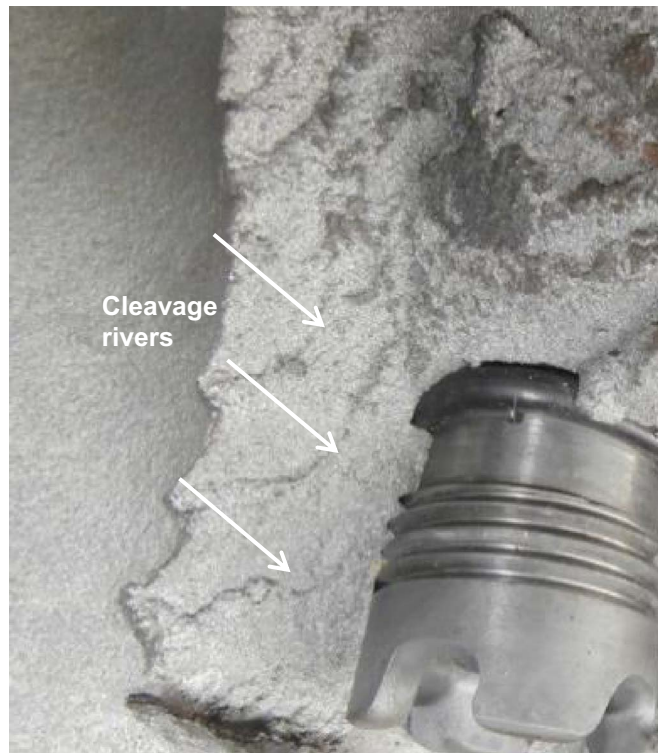
Fig. 4. Fracture surface, cleavage marks in the last part of fracture propagation.
