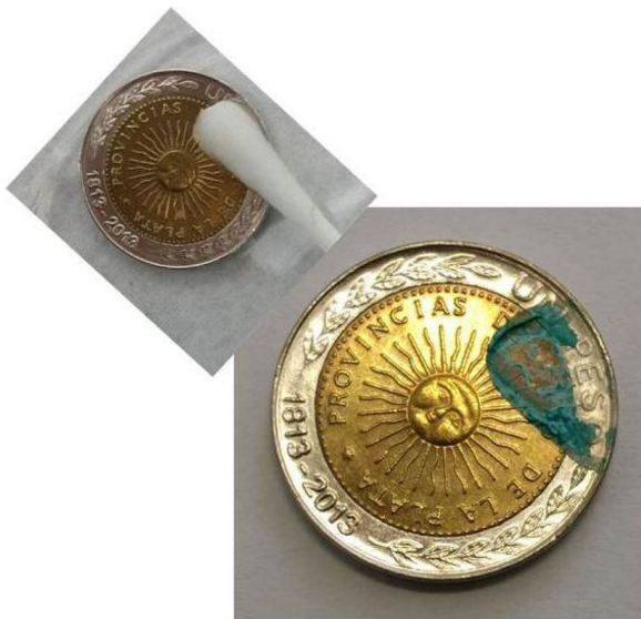
Fig. 8. Photo of a 1-peso coin before and after exposure to the artificial sweat.
