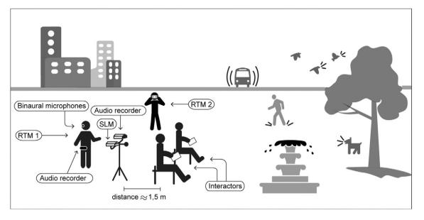
Fig. 3. Layout of the data collection scene in the environment, including the suggested position and orientation of the research team members (RTMs) and the instruments.
