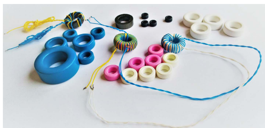
Fig. 4. Toroidal ferrite magnetic cores. Shown are insulated commercial Mn-Zn ferrites (blue toroids) and Ni-Zn ferrites (pink, white) along with uncoated ferrites (black) of both types. Two insulated Ni-Zn toroids and one uncoated Mn-Zn toroid are prepared with primary (inner) and secondary (outer) windings for fluxmetric measurements.
