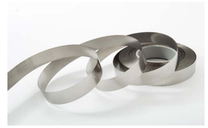
Fig. 7. Ribbon of amorphous soft magnetic alloy. Thin (5 to 50 \mu\text{m} ) ribbons of amorphous alloys are produced by planar flow casting.
