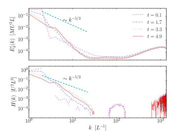
FIG. 13. (Color online) Spectra of the incompressible kinetic energy and of the helicity at  $T = 0.64T_{\lambda}$  in the simulation with N = 4096 at different times. A turbulent scaling law is shown as a reference. Although nonlinear excitations develop, the range of scales compatible with the turbulent scaling is short and at late times the spectrum decays rapidly.
