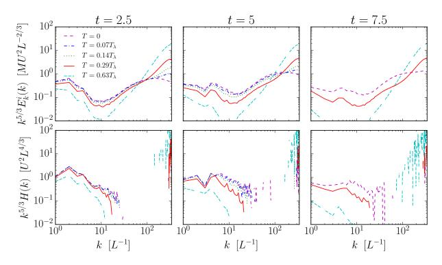
FIG. 12. (Color online) Compensated version of the incompressible kinetic energy and helicity spectra shown in Fig. 11. As seen in the figure, only at the smaller temperatures some range of wave numbers compatible with  $k^{-5/3}$  scaling (i.e., an approximately flat compensated spectrum) is recovered.
