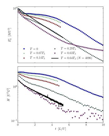
FIG. 7. (Color online) Evolution of the incompressible kinetic energy (top) and of the helicity (bottom) as a function of time and at different temperatures in semi-logarithmic scale. All simulations have N = 1024, except the one indicated with the solid black line which has N = 4096. At the highest temperatures quantities decay exponentially in time.
