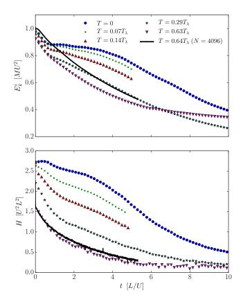
FIG. 6. (Color online) Evolution of the incompressible kinetic energy (top) and of the helicity (bottom) as function of time at different temperatures. All simulations have N = 1024 linear resolution, except the the one indicated with the solid black line which has N = 4096. The early "inviscid-like" behavior seen at low temperature, in which energy and helicity remain approximately constant, is lost as the temperature is increased.
