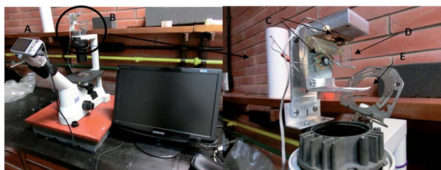
Fig. 1 Picture of the setup used as an interface for transmission measurements of different systems. (Left) (A) camera; (B) illumination system. (Right) Zoom picture of the illumination system (C) LEDs; (D) dichroic mirror; (E) homemade diaphragm.
