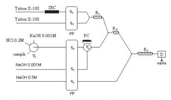
**Figure 1**. PP: peristaltic pump;  $V_1$ : six way valve;  $V_2$ : injection valve;  $q_1$ : Triton X-100 flow rate;  $q_2$ : diluent flow rate;  $q_3$ : HCl, sample and NaOH flow rates; SRC: solid reagent column; PC: preconcentration column;  $R_pR_2$ and  $R_3$ : reactors; D: detector; W: waste
