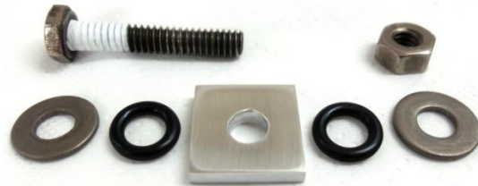
Figure 1. Aluminum specimen (center), rubber O-rings and titanium bolt, nut and washers used for assembling creviced specimens.
