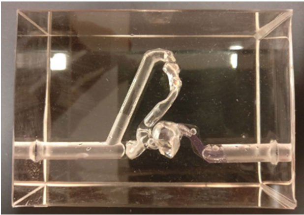
Fig. 2 Patient-specific silicone model of the aneurysm of the left internal carotid artery
