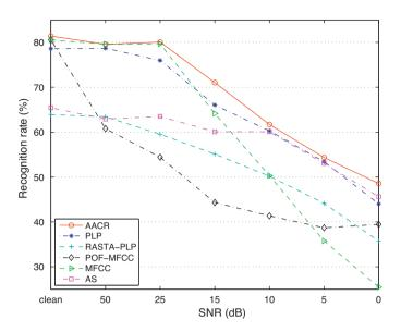
Fig. 7. Recognition rates in percent for the classification of the 5 phonemes in the presence noise at different SNR, from clean speech up to same energy levels of speech and noise (SNR = 0 dB).
