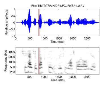
Fig. 3. Principal signals in the process of obtaining the spectro-temporal patterns: sonogram (top) and auditory spectrogram (bottom). A section corresponding to the sliding window, from which each spectro-temporal pattern is generated, has been marked with vertical lines.
