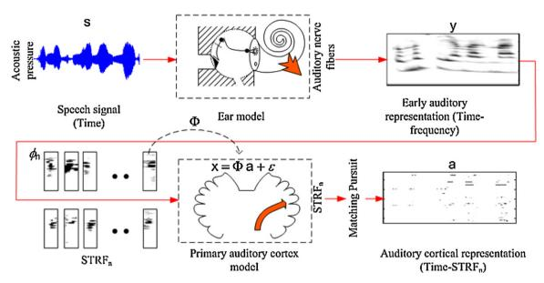
Fig. 2. Schematic diagram of the method used for estimating the approximated auditory cortical representation (AACR).
