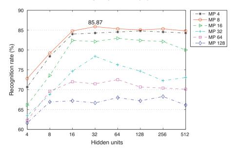
Fig. 6. Initial tuning of the number of selected coefficients in the algorithm and hidden units in the neural networks. The best performance is obtained for 8 selected coefficients and 32 nodes in the hidden layer of the MLP.
