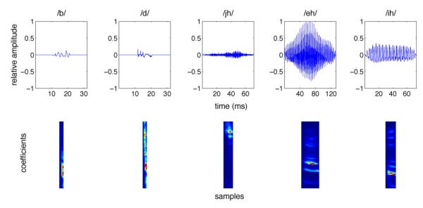
Fig. 4. Examples of the five phonemes used in the experiments showing the sonogram (top) and their respective auditory spectrogram (bottom). The spectrograms have 64 frequency coefficients in height from 0 to 8 kHz and a minimum of 4 coefficients in length, as it can be seen in the shortest phonemes.
