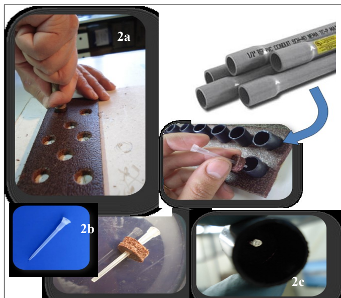
Fig. 2. Device construction. 2a) Perforating the plastic base with a punch. 2b) Entire tip and truncated tip with foam plug. 2c) Capsule from inside.
