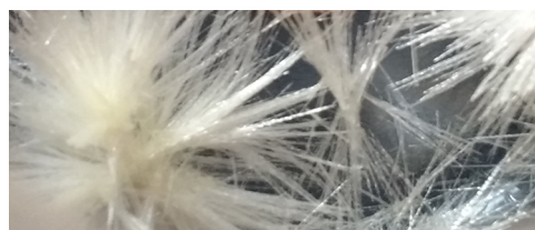
Figure 6. Needle-like crystals of S-fa obtained after purification by recrystallization.
