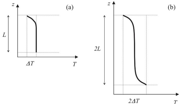
Fig. 12. The average temperature distributions corresponding to the experimental setup used here (a) and that of Rayleigh–Benard’s (b).
