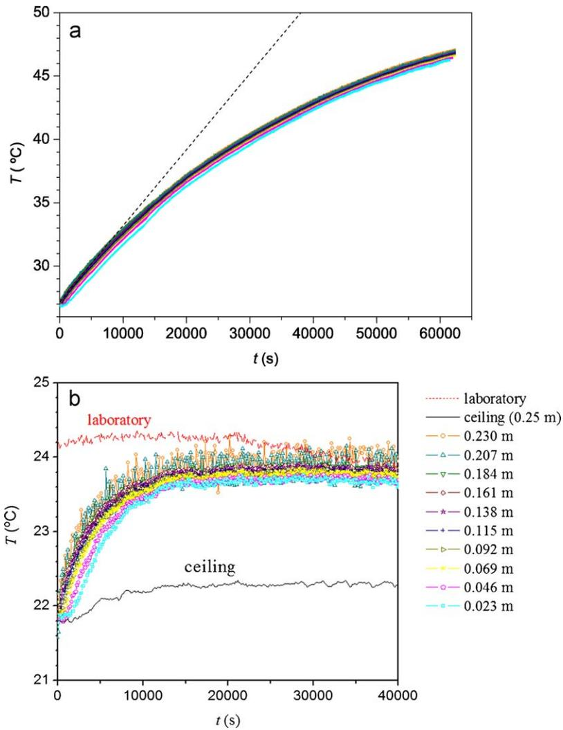
**Fig. 4.** (a) Evolution of the temperature at different height from the floor in the laboratory model with insulated top and a 60 W heater. The dashed line corresponds to the evolution of the expected mean temperature in a model without heat losses. (b) Evolution of the temperature at the cooled ceiling, ambient and at different heights in the fluid bulk for the experiments showed on the right of Figs. 2 and 3.
