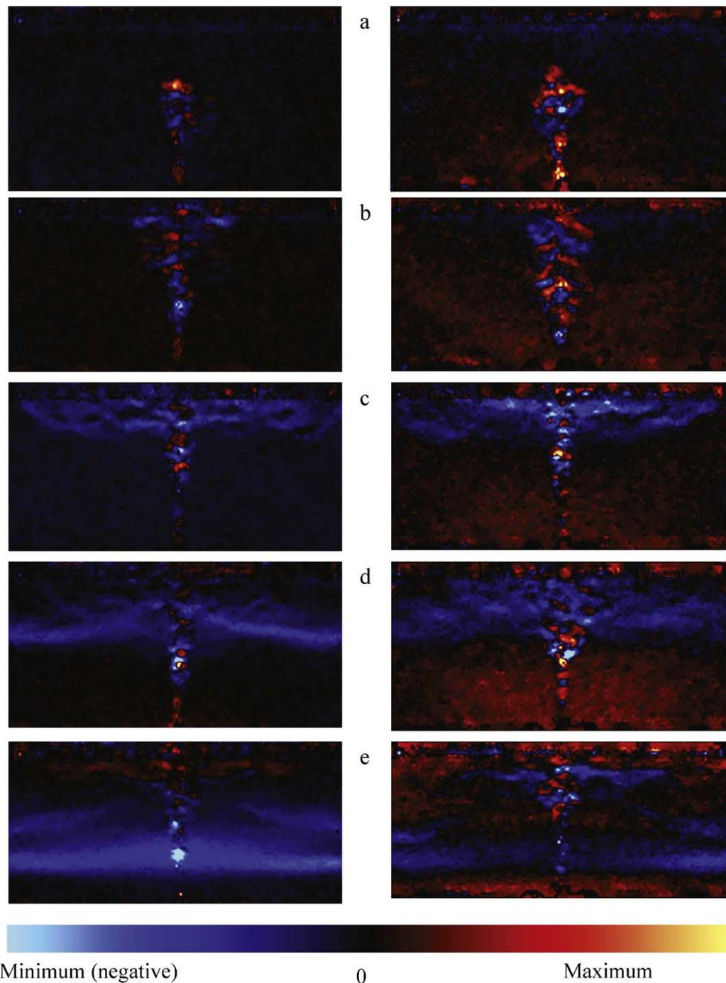
**Fig. 3.** Vertical component of the de temperature gradient corresponding to the same images shown in Fig. 2 for the insulated top box (left) and the cooled-ceiling system (right).
