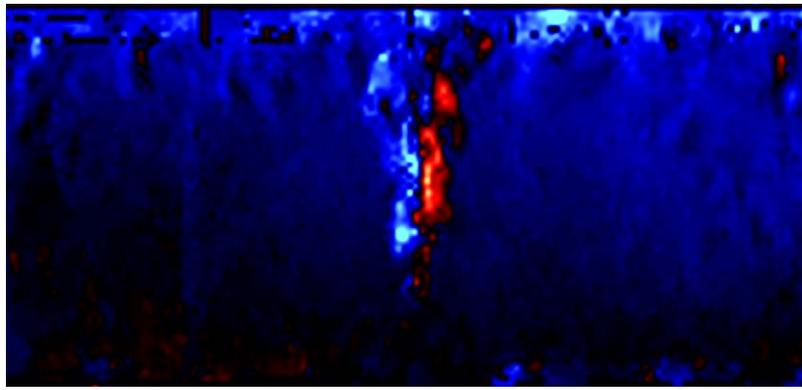
Fig. 10. Distribution of the horizontal component of the temperature gradient obtained by applying synthetic schlieren during the steady state.
