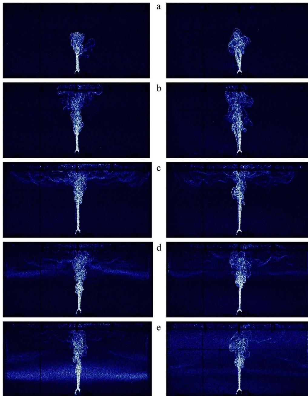
**Fig. 2.** Images obtained with synthetic schlieren at (a) 20 s, (b) 40 s, (c) 90 s, (d) 250 s and (e) 800 s after the 60 W heater is turn on for the cases in which the upper contour is insulated (left) and at constant temperature (right).
