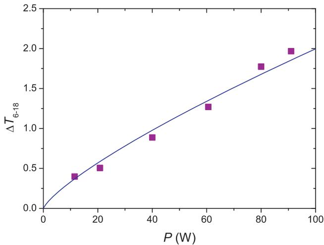
Fig. 7. Difference between the average of the temperatures measured with the thermocouples located between 0.069 and 0.184 m within the fluid, and  $T_{top}$  during the steady state regime. The line represents Eq. (7).
