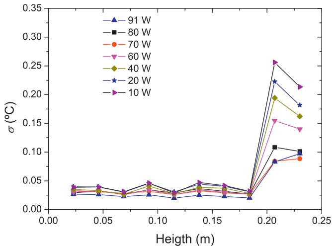
Fig. 8. Standard deviation  $\sigma$  of the time average of the temperature measurements shown in Fig. 4b.
