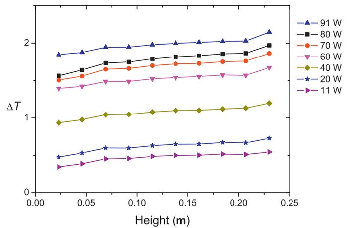
**Fig. 6.** Difference between the average  $\langle T \rangle$  of the temperatures measured by the thermocouples immersed in the fluid at the height indicated in abscissas and the CC temperature  $T_{cc}$  during the steady state. The corresponding power values are indicated to the right of the figure.
