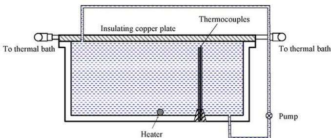
Fig. 1. Schematic of the laboratory physical model.
