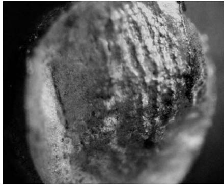
Fig. 11. Typical SEM fractographs of aluminium samples submitted to tensile strength.
