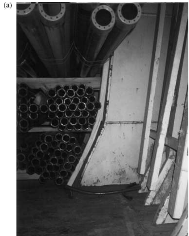
Fig. 2 Storage of pipes during shipping. (a) typical lateral protection by wood sticks, (b) common hits during loading.
