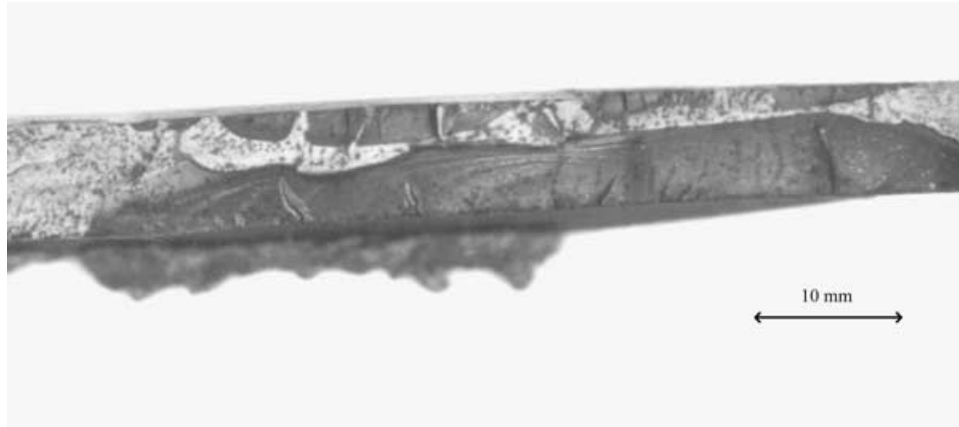
Fig. 1 Typical fracture surface due to transit fatigue (TF) in a seamless pipe.
