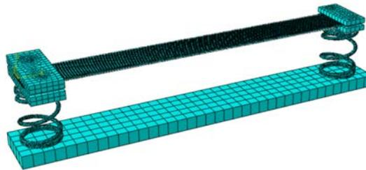
**Figure 5.** Abaqus 3D model of the harvesting device.
