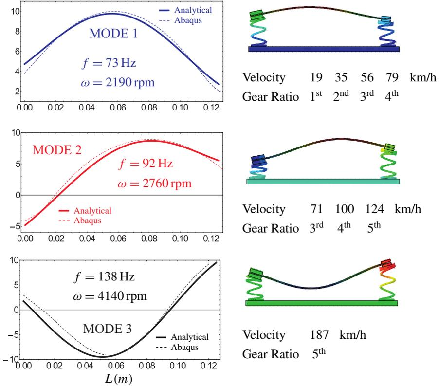
**Figure 6.** First three flexural mode shapes: comparison between the analytical and computational models.
