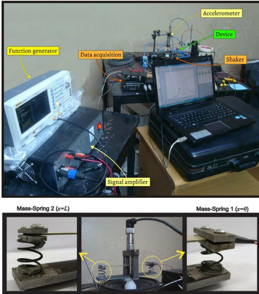
**Figure 7.** Experimental setup. Top: general scheme. Bottom: detailed view showing the shaker, the device and the accelerometer.
