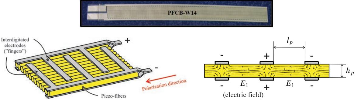
**Figure 2.** Schematic view of the piezofibers composite. Top: real piezofiber composite PFCB-W14 from Advanced Cerametrics Inc. (168 fingers). Left: geometric detail of only four “fingers” of the electrodes. Right: cross-sectional view of the fibers and electrodes showing the generated electric field.
