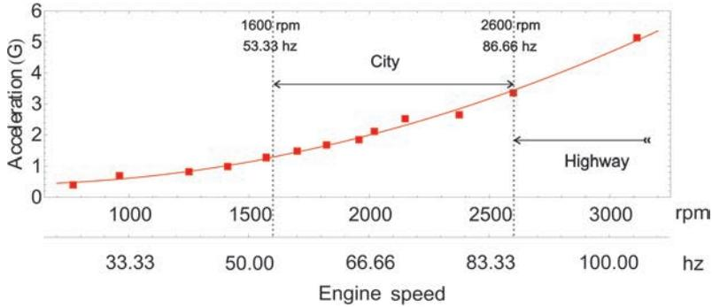
**Figure 10.** Engine acceleration level based on rpm.
