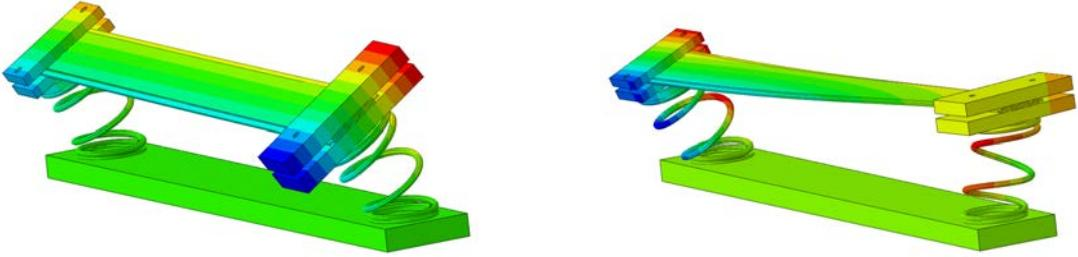
**Figure 9.** Additional three-dimensional modes generated using Abaqus that were not included in the analytical model. Left: first mode (lateral). Right: third mode (torsional).
