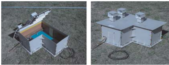
Figure 4. Scale model of the analysed building. Inner view: reproduction of the surface reflectances. Outer view: reproduction of the light pipes layout.
