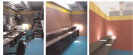
Figure 7. Visual presentation of the three rooms analysed. Real situation, scale model picture and image captured by DiaLux.
