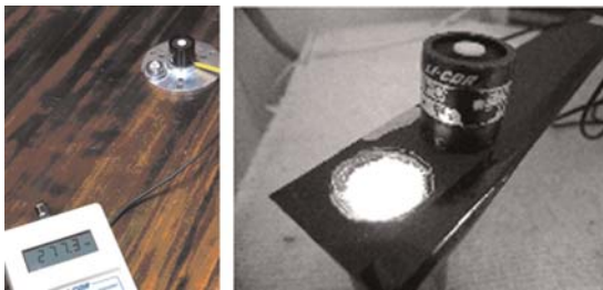
Figure 3. LI-COR 189 radiometer and LI-210 SB photometric sensor.
