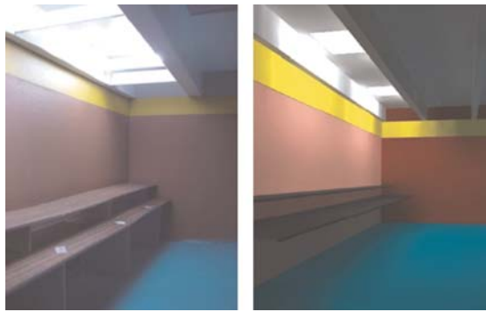
Figure 11. Site appearance with natural lighting system on 21 September. (Left) Scale model with diffuser; (right) Virtual scale model with diffuser.
