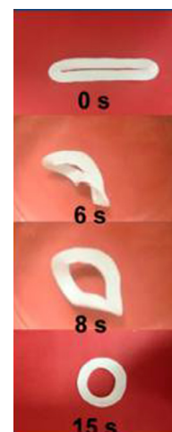
Fig. 7. Recovery of a temporary compressed ring to the initial shape when heating at 60 °C. Reprinted with permission from Bilici et al. [27].
