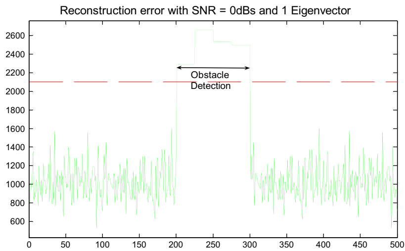
Fig. 18. Reconstruction error when the section of track is not free.
