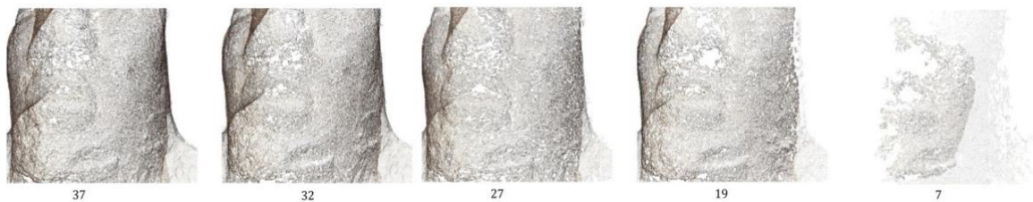
Fig. 5. Point clouds generated by VisualSFM + CMVS with different sets of images in order to determine the required overlap to achieve a denser point cloud. 37, 32, 27, 19 and 7 were the number of images in each set, decreasing the overlap.
