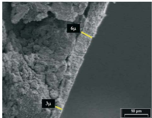
Figure 3. SEM photograph of the external surface of catalyst C3T (2000×).
