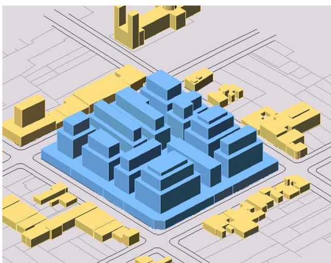
Fig. 12. Outline of analyzed block of buildings, maximum density possible according to the CUE of the Capital City.
