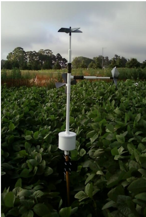
Fig.2. UVW anemometer. Photograph by María Gassmann
