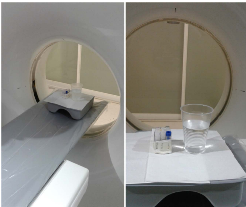
Fig. 1. Pack containing irradiated and non-irradiated vials of Fricke, PAGAT, NIPAM and ITABIS dosimeters along with water and aluminum samples for CT scanning.
