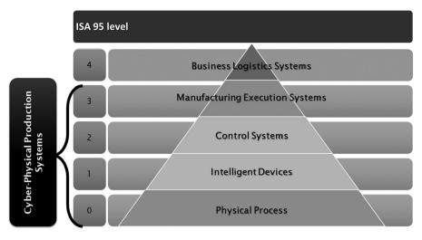
Figure 3. Levels of ANSI/ISA95 integrated into CPPS.
