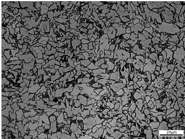
Fig. 1—Bright field OM micrograph showing the as-received DP steel microstructure.
