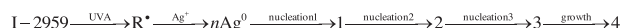
Scheme 1. Sequential nucleation-aggregative growth model for the reductive synthesis of AgNPs by UVA-photolysis of I-2959 as source of ketyl radicals ( \text{R}^{\bullet} ).
