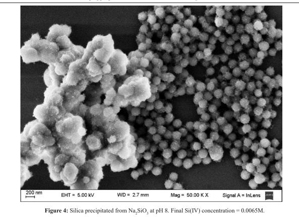
If the pH is buffered at a value around 8, big aggregates are obtained, mixed with spheres of circa 100 nm of diameter (Figure 4).
