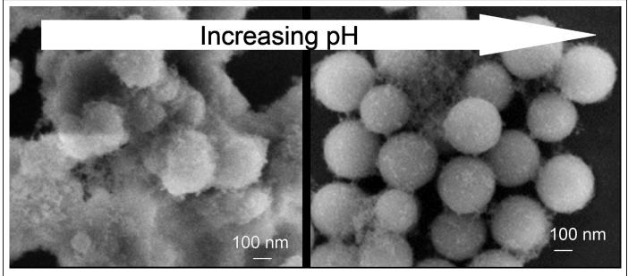
Figure 2: SEM images of empty silica nanoparticles synthesized at constant [Si] with variable pH without microemulsion.
