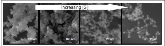
Figure 7: SEM images of silica nanoparticles synthesized at constant pH with variable [Si] with microemulsion.
