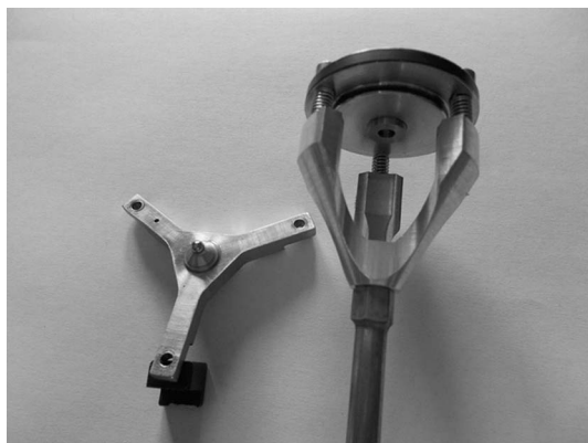
FIG. 4. Ball and basket support of pendulum.
