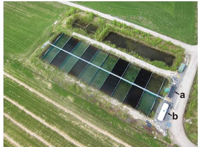
Fig. 1 Aerial picture of EXEF (Umeå University Experimental Ecosystem Facility). The pond system (73 m long, 25 m wide) is divided into 20 sections (12.5 × 7.3 m, 1.49 m average depth). The facility allows for warming with heat exchangers (a), and manipulations of input water characteristics; in (b) is shown the tank where the humic river water is stored
