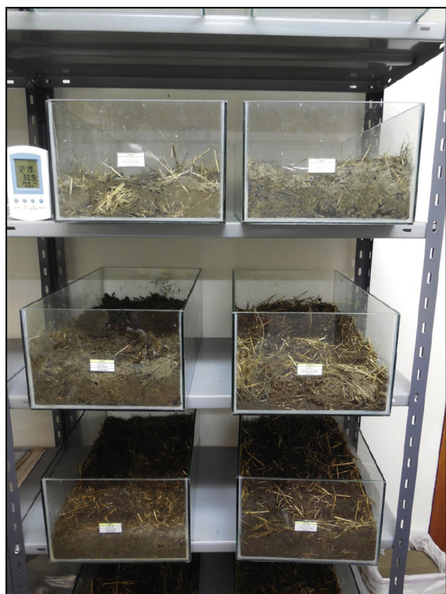
Fig. 1. Biobeds at laboratory scale.
