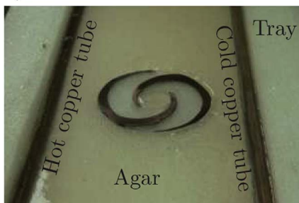
Fig. 7. Experimental heat flux inversion: a) hand-made device; b) domain of analysis; c) experimental setup.
