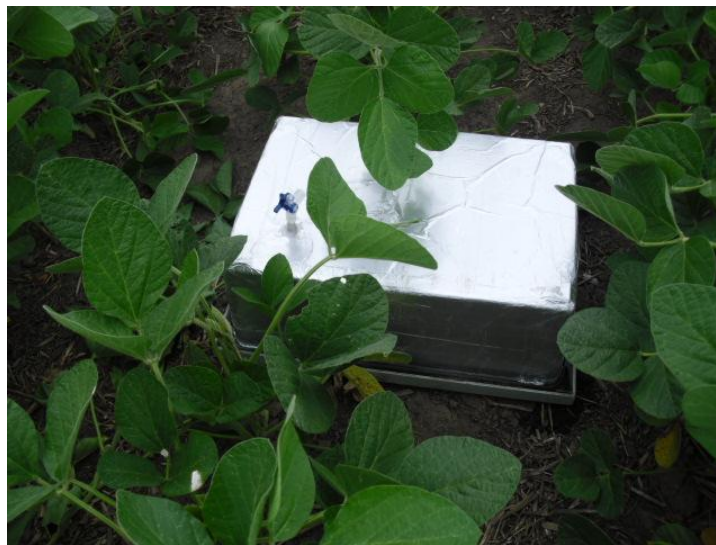
Figure 3: Non steady-state chambers used by the Institute of Climate and Water (INTA Argentina) on a soybean field.
