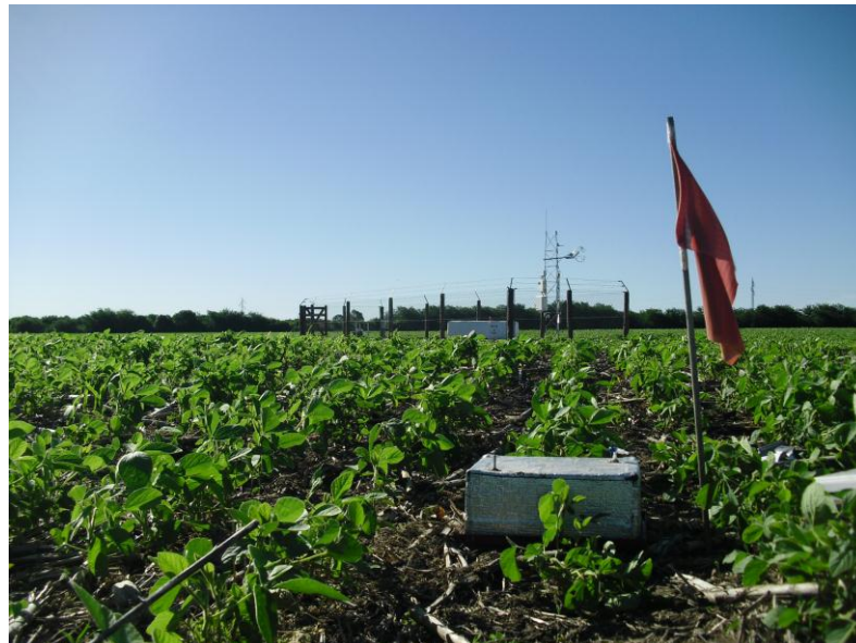
Figure 6: Field site 2, where eddy covariance (CO 2 , N 2 O and water vapour) and non steady-state chamber (N 2 O) measurements are carried out.
