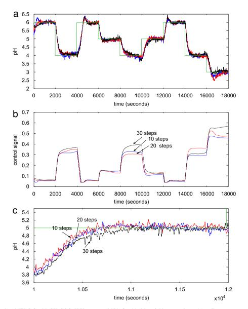
Fig. 13. Online application MFLC for NaCH<sub>3</sub>COO-HCl systems, MSA for 10, 20 and 30 step-actions: (a) online responses, (b) control signal and (c) systems for 10000-12000 s.
