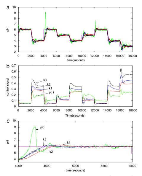
Fig. 12. Online application MFLC for NaCH<sub>3</sub>COO–HCl systems, Q-learning standard for  $k_1 = 1 \times 10^{-5}$ ;  $k_2 = 2 \times 10^{-5}$ ;  $k_3 = 3 \times 10^{-5}$  and compare to PID: (a) online responses, (b) control signal and (c) systems for 4000–6000 s.
