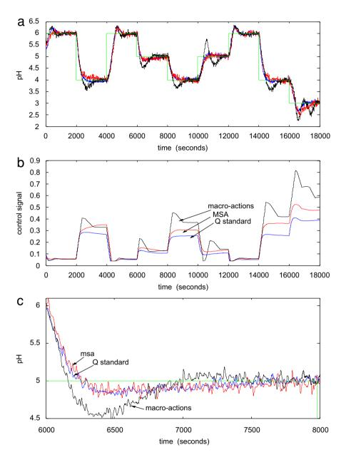
Fig. 14. Online application MFLC for NaCH<sub>3</sub>COO-HCl systems, macro-actions: (a) online responses, (b) control signal and (c) systems for 6000-8000 s.
