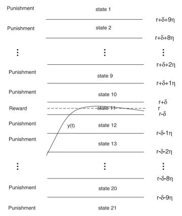
Fig. 7. State definition and control objective and definition of states: dash line presents a reference.
