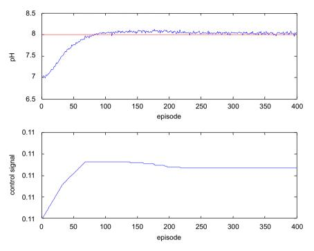
Fig. 4. Responses and control signal of strong acid-strong base system.
