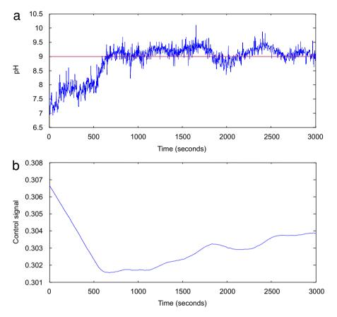
Fig. 16. Online application of MFLC for NaOH-HCl systems: (a) responses and (b) control signal.
