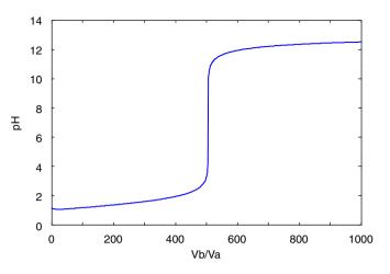
Fig. 3. Titration curve strong acid-strong base system of the model.
