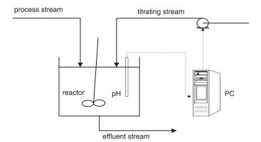
Fig. 10. pH neutralization process plant.
