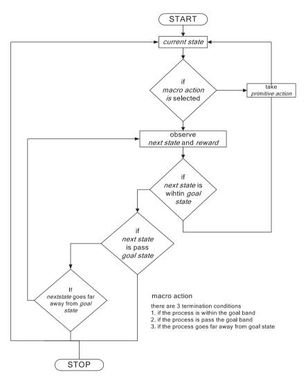
Fig. 9. Implementation of macro action and definition of termination conditions.
