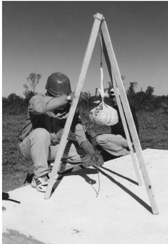
Fig. 2. Placement of the explosive charge suspended above the slab.
