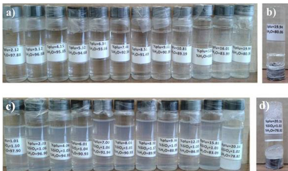
Fig. 1. a) Pluronic F-127 aqueous solutions with weight fractions in the 2–20 wt% range. Notice that the viscosity of the solutions increases with the weight fraction of Pluronic F-127. b) Detail of the solution with Pluronic F-127 weight fraction ~ 20 wt%. c) Mixed dispersions containing fix silica nanoparticles concentration (~ 1 wt%) and increasingly amounts of Pluronic F-127 (2–20 wt% range). Notice that the increase of Pluronic F-127 weight fraction leads to an increase on the viscosity of the dispersions. d) Detail of the mixed silica nanoparticles - Pluronic F-127 dispersion containing a weight fraction of copolymer ~ 20 wt%.
