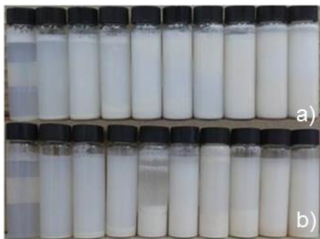
Fig. 3. Dispersions of eugenol in aqueous Pluronic F-127-decorated nanoparticles (Pluronic F-127 2 wt% and silica nanoparticles 1 wt%) with increasingly eugenol concentrations (from left to right: 1–10 wt%): as prepared (a) and after 48 h (b). The values of R_{\text{plu/eug}} represented (from left to right) are: 1.56, 0.86, 0.65, 0.46, 0.37, 0.31, 0.26, 0.22, 0.20 and 0.18.
