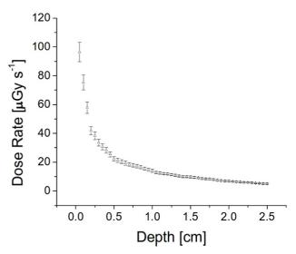
FIGURE 2. Monte Carlo results for the in-depth dose rate for homogeneous (tissue-equivalent) phantom irradiated with the *in-vivo* X-ray fluorescence scanning device.
