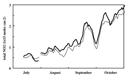
Fig. 4. Total vertical column of NO<sub>2</sub> measured at morning twilight (thinner line) and evening twilight (thicker line) by the INTA/DNA UV–vis zenith-sky spectrometer at Marambio ( $64.2^{\circ}$ S), smoothed by a 5-day running mean. As discussed in Section 3.1, these measurements show rather more NO<sub>2</sub> near midwinter than in the early 1990s at Faraday, only 1.1° further south.
