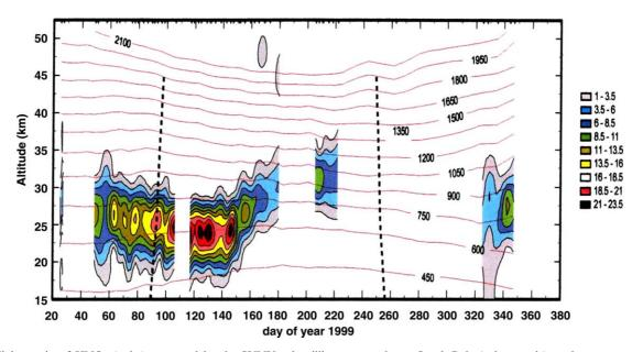
Fig. 7. Mixing ratio of  $HNO_3$  (ppbv) measured by the SUNY sub-millimetre sounder at South Pole (colour scale), and contours of potential temperature (K) from South Pole radiosondes supplemented by NCEP analyses above balloon limits (lines). The enhancement of  $HNO_3$  in the upper stratosphere beginning just before the break in data beginning on day 177 is similar to enhancements observed more completely when the sounder was deployed in 1993 and 1995, as discussed in Section 3.6.
