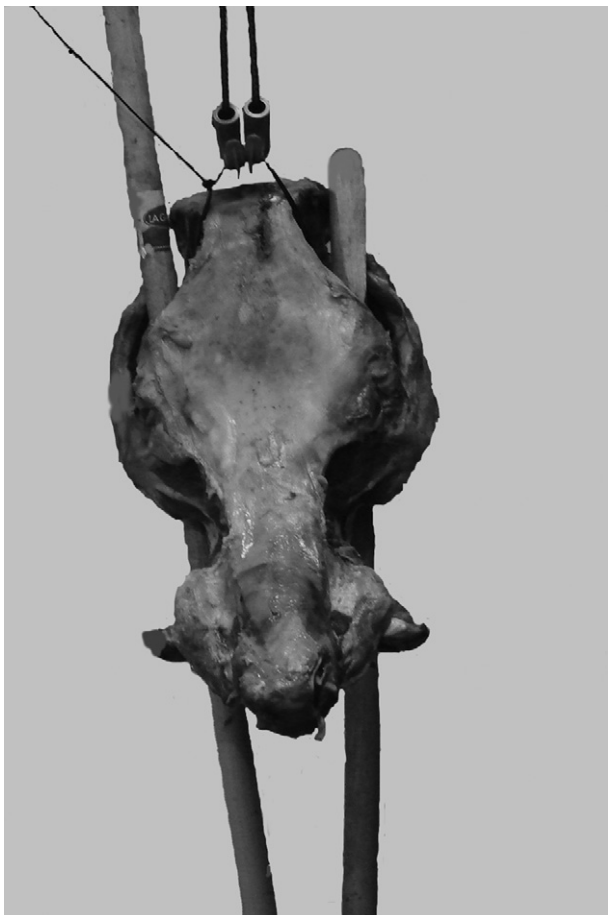
Fig. 2. Positioning of swine skulls in order to be impacted.
