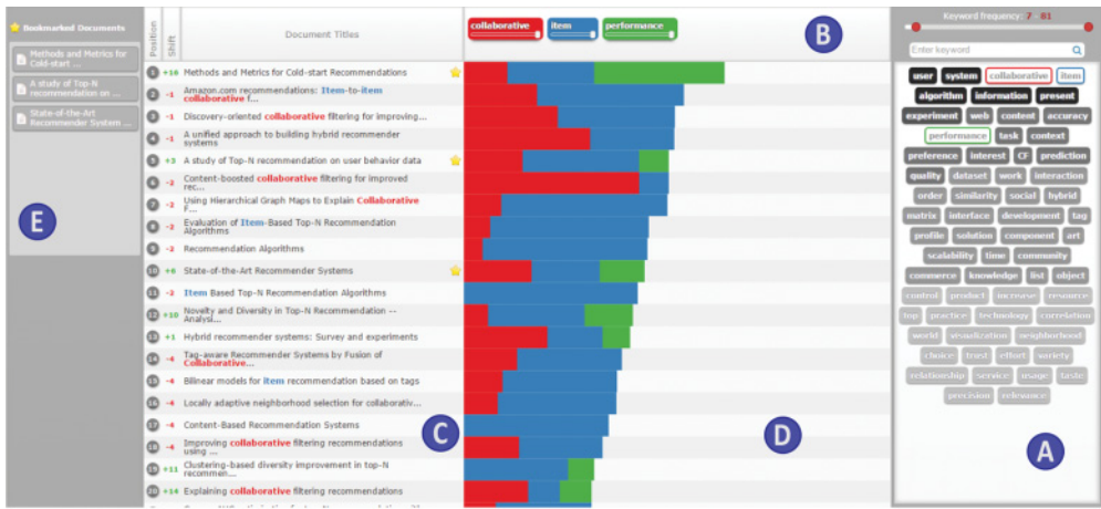
Fig. 3. uRank user interface displaying documents related to recommender systems , with ranking updated to match the keywords “collaborative,” “item,” and “performance.” A. The Tag Box presents a keyword-based summary of the document collection. B. The Query Box contains keywords selected by the user. The Document List (C) and the Ranking View (D) present a list with augmented document titles and stacked bars indicating relevance scores. E. The Bookmark Overview shows bookmarked documents.
