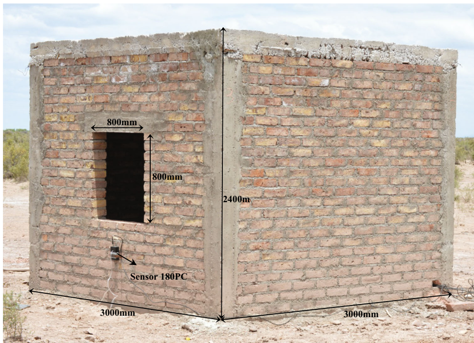
Fig. 1 Room for experimental tests
