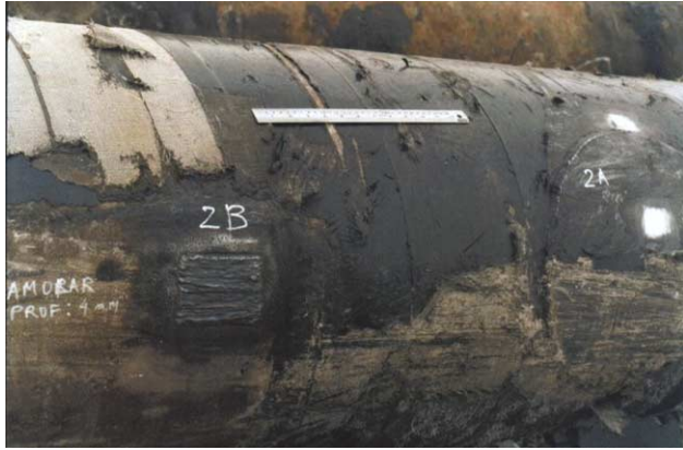
Fig. 5. Circular patch and weld repair of artificial defect in pipe 2.
