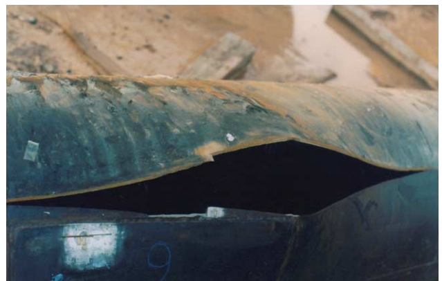
Fig. 8. Final fracture in test of pipe 6.
