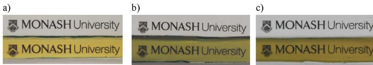
Figure 5. Photographs of cured 1.4 mm thick specimens (located at the bottom of the images) on top of a white printed card, indicating the level of transparency of (a) polymerized TetMESi, (b) polymerized TetMESi after hydrolysis with water vapor, and (c) polymerized TetMESi after hydrolysis and drying.
