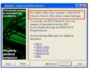
Fig. 6–10: Required steps for accessing to the Aspen Plus V 7.2 recommended packages.
