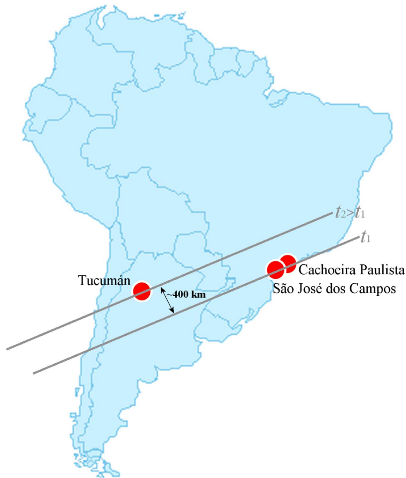
Figure 11. Wavefront of a medium-scale traveling ionospheric disturbance propagating northwest in the Southern Hemisphere at time t_1 and time t_2 > t_1 .
