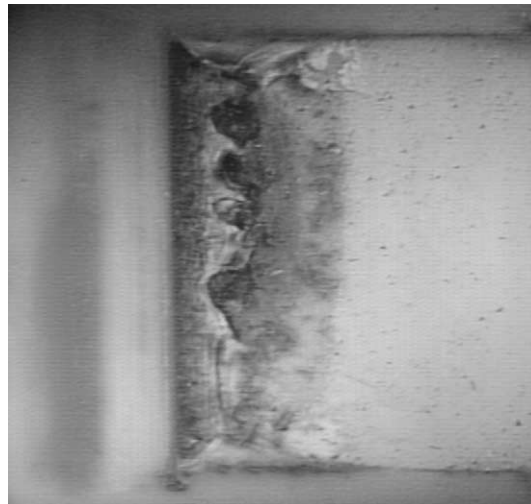
Fig. 10. Photograph of the fracture surface of a PE2 polyethylene sample painted prior to complete fracture (The crack extended from the left to the right.).
