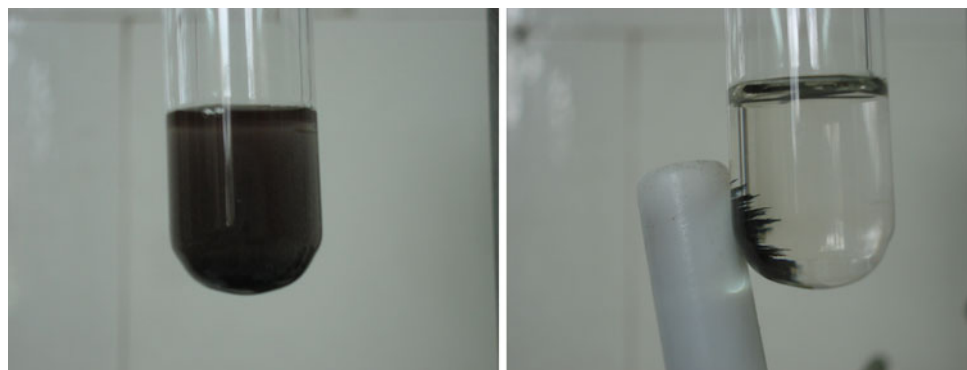
Fig. 3 CuFe 2 O 4 catalyst during reaction, under stirring and removal by external magnet
