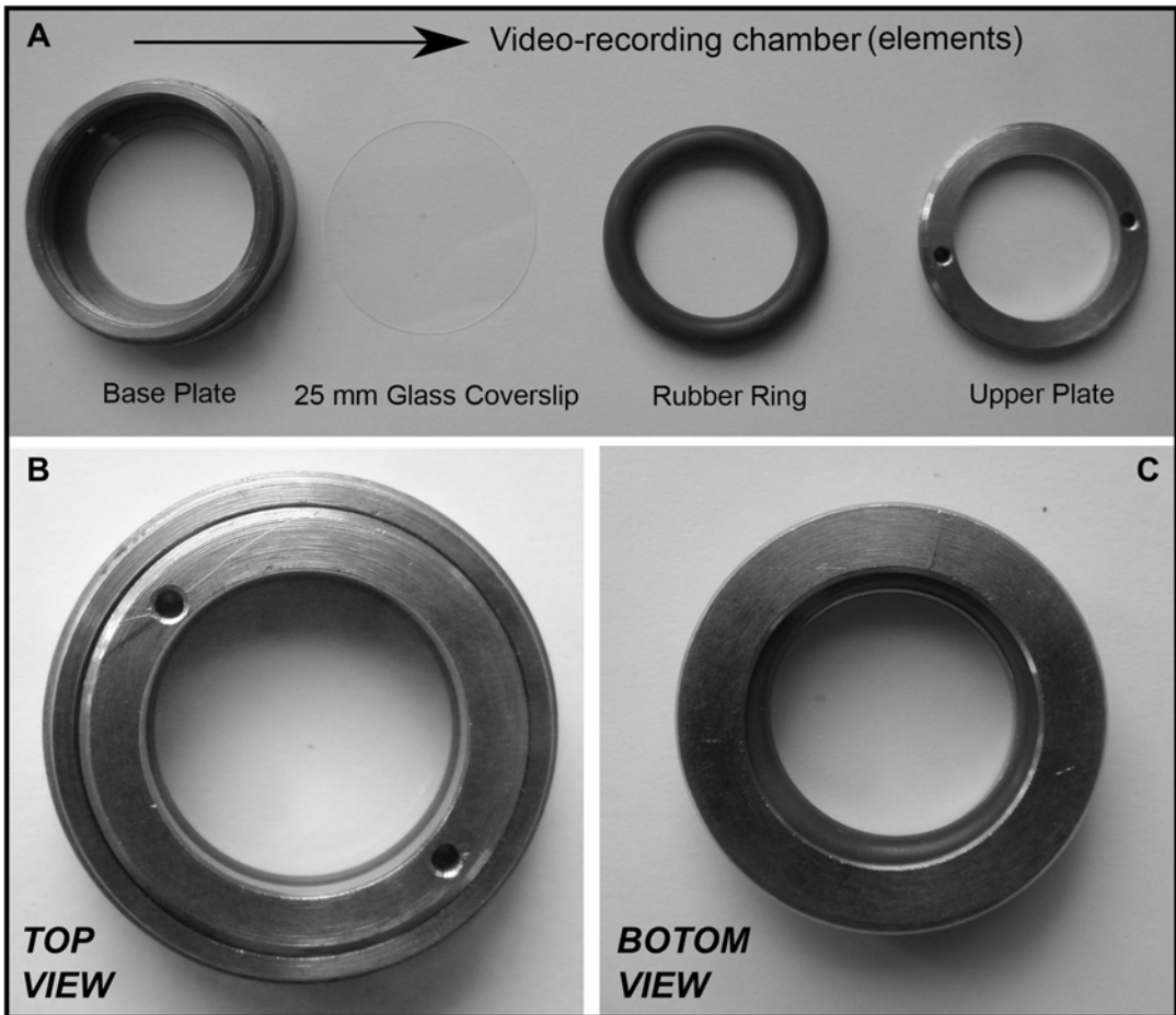
Fig. 1 (a) Components of the open chambers used for video recordings. They include: (a) base plate; (b) 25 mm coverslips, where the cells are grown; (c) a rubber ring, and (d) the upper plate. (b) Top view of the assembled chamber. (c) Bottom view of the assembled chamber
