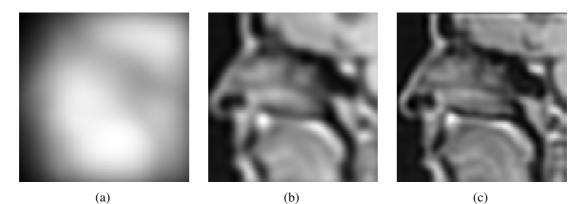
Figure 1: 1(a): Blurred image (data for the inverse problem); 1(b): Regularized image obtained with the Tikhonov-Phillips method of order 0 (TP0); 1(c): Regularized image obtained with the Tikhonov-Phillips method of order 1 (TP1).
